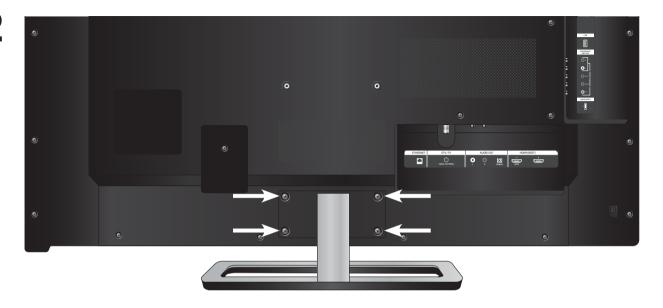
Align the stand with the back of the TV. Use a Phillips screwdriver to insert and tighten the four (4) included M6 x 18mm Phillips screws into the holes on the back of the TV.
